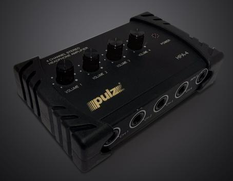
Pulz HPA-4 is a stereo headphone amplifier with possibility of connecting 4 headphones at the same time and each output volume can be controlled individually. Input and Output connectors for this unit are 6.3 mm stereo headphone jack. The unit works on a 12V DC 200mA supply adaptor which is included in the box.
